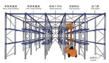
This type is specially designed for storage of large quantity of goods of one kind, consists of a continuous block of racking not divided by aisless and there are two type: one side drive-in and two-way drive-in.
